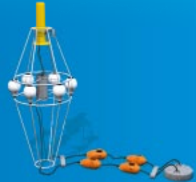
PAM The Passive acoustic monitoring (PAM) detects marine mammals by monitoring their vocalizations. The array of hydrophones (orange) listens to establish the presence of mammals. The radar beacon (yellow) makes it visible to ship traffic.
